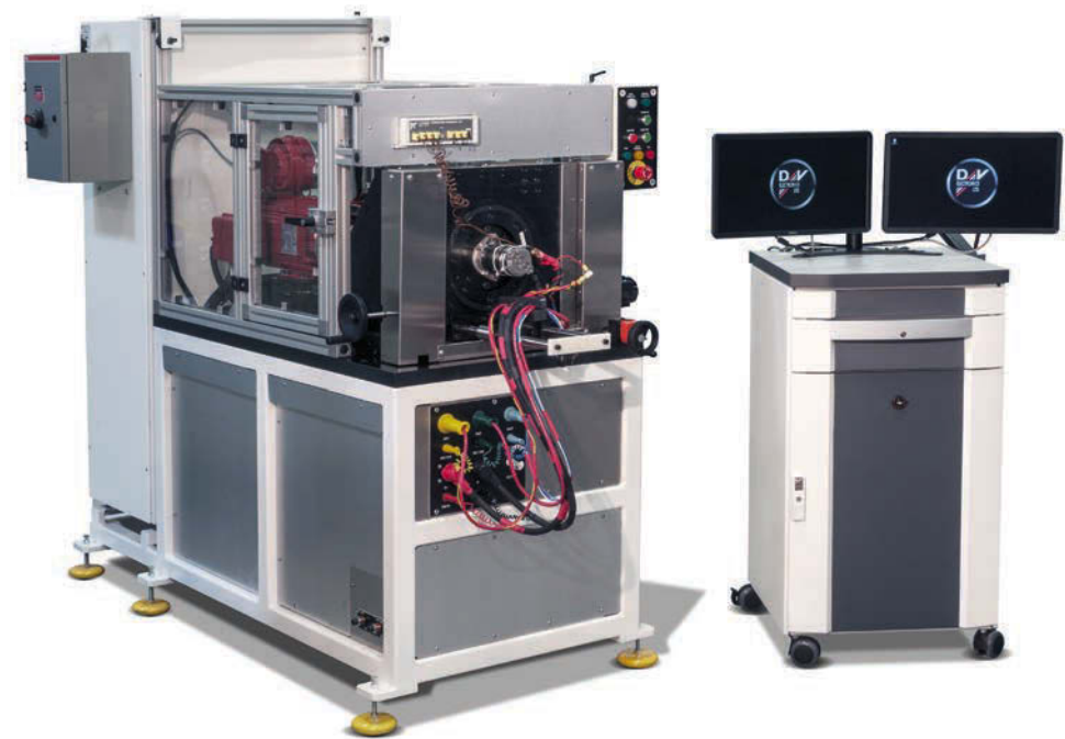
ABOVE: The improved ST-64 G2 bench for testing all types of starter motors
