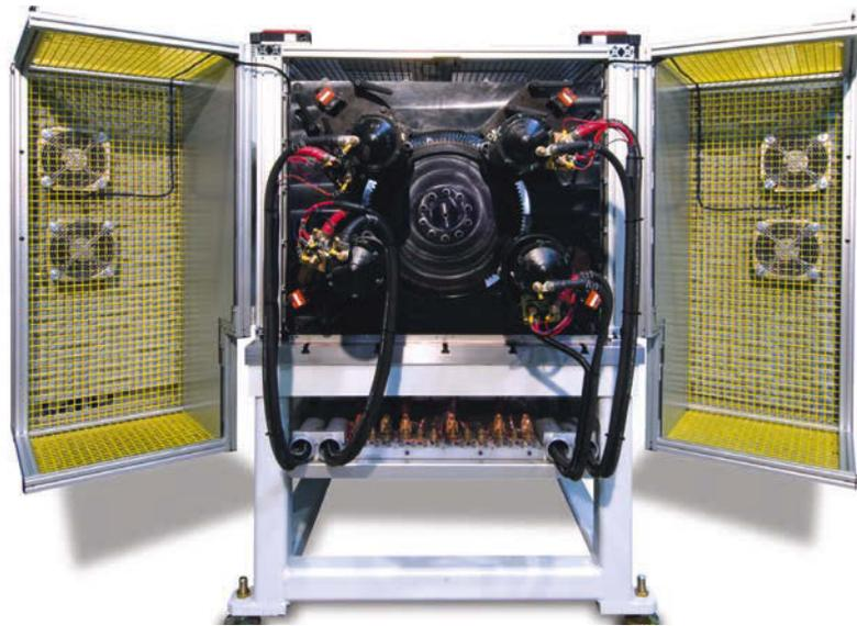
millions of cycles, which is impossible to duplicate on a live engine test stand. It can also be used in a variety of applications from starter design validation to flex plate durability verification.
