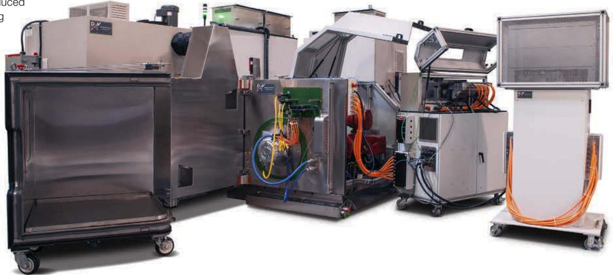
The EPT-130 platform was developed to run demanding lifetime testing for a switch reluctance electric motor and inverter
