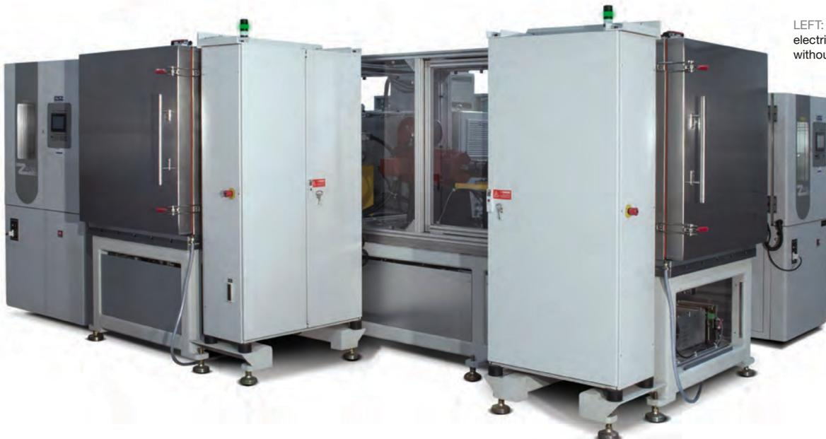
LEFT: VSM-100 enables electrical system tests without the full vehicle
